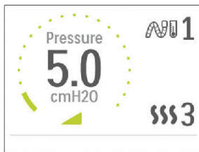
Ramp Pressure Screen
